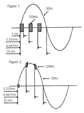
Note. - For clarity, the signals in figure 1 are shown as they would be seen through a high pass filter. The 5 0 Hz. waveform is only shown for reference. In reality the signals are actually superimposed on the 5 0 Hz. waveform and look more like that shown in figure 2.
