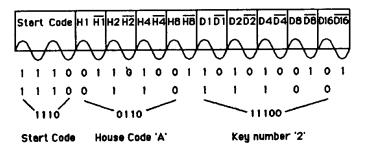
The Tables in figure 5. show the Binary Codes to be transmitted for each House Code and Key Code. The Start Code is always 1110 which is a unique code and is the only code which does not follow the true complement relationship on alternate half cycles.
